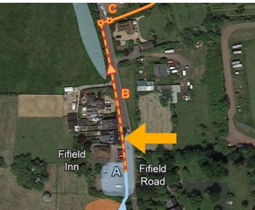
**Wet Spot 7B** from south of the Fifield Inn northwards to the same chamber at Garden Cottage has been dysfunctional for a very long time. The problem starts at the pipe under the entrance to the pipe car park which simply has inadequate capacity and backs up eventually into the car park as seen many times and shown below.
